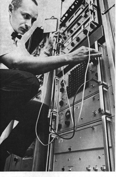
EPOCH TIME or the time when an event occurred can be retrieved from reco test data with this IRIG Timer (Inter Range Instrumentation Group). Gene Medina (7331) records readouts from the device which is equipped with tape search and playback capability. IRIG can locate events in time down to milliseconds.
